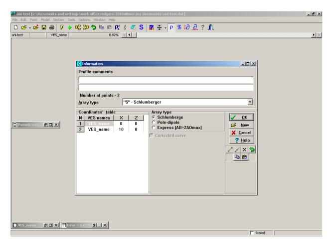
Information window will appear. N column on Coordinate Table is number of joined VES point. VES names column is name of each VES point (can be changed by clicking the VES\_name in VES names column). X is distance between united VES points and Z is elevation of each VES points.
