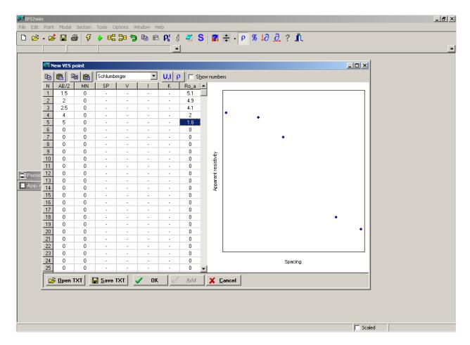
Data are inputted in column by clicking the column. After data were inputted, points will be plotted in a graph beside the VES column, then click OK button.
