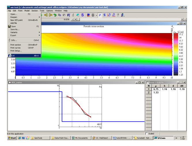
For joining another VES data, Restart IP 2 Win software by close the software and re run it.
