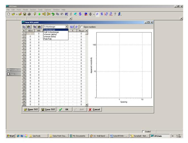
Choosing electrode configuration is important before inputting data, as example Schlumberger's electrode configuration was chosen.
