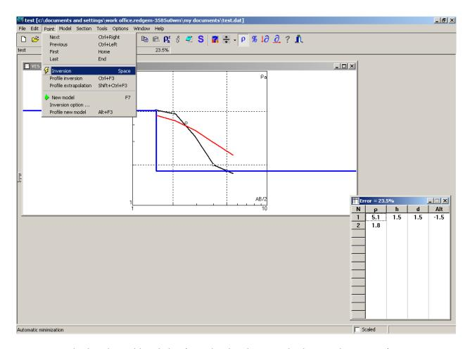
Data error is displayed on table title bar (error level in the example above is about 23.5%). Data error can be corrected automatically by clicking Point>Inversion. Manual data correction can be done by dragging the curve.
