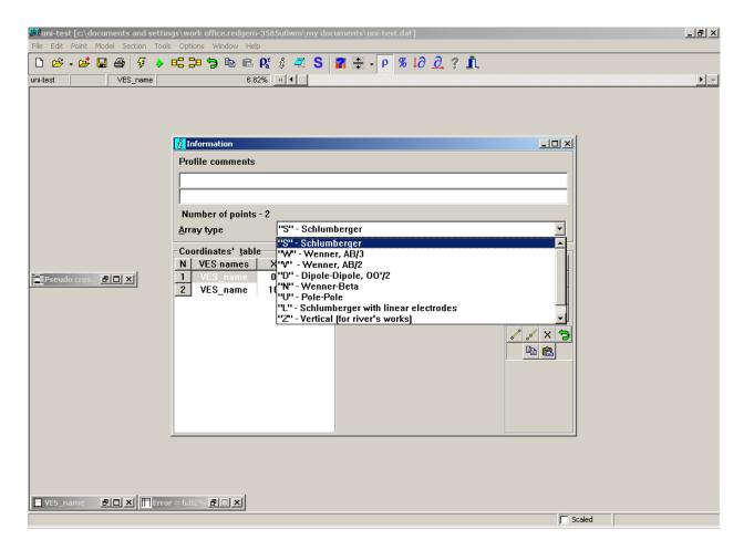
Choose Array type from the joined data as example Schlumberger (Chosen array must be same as the first chosen electrode configuration). Click OK button.
