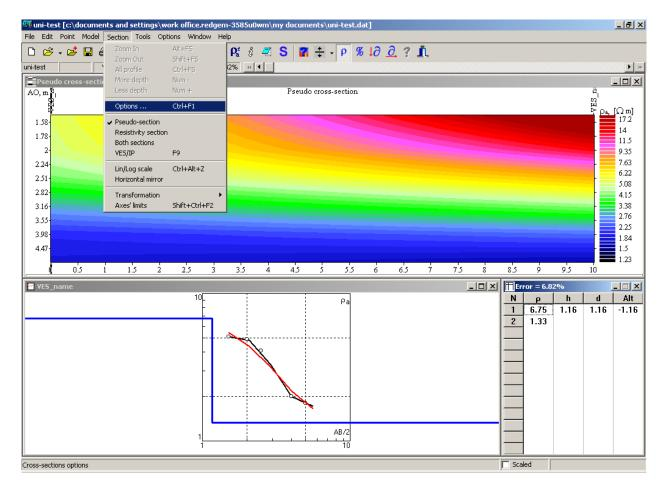
Pseudo Cross Section and Resistivity Cross Section display can be set by clicking Section>Options.
